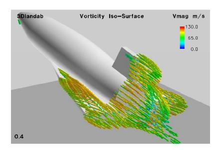
Description: Two step simulation: a) SS solution a 100 m/s, b) transient solution with approximate landing movement
