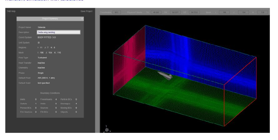
Description: Two step simulation: a) SS solution a 100 m/s, b) transient solution with approximate landing movement
